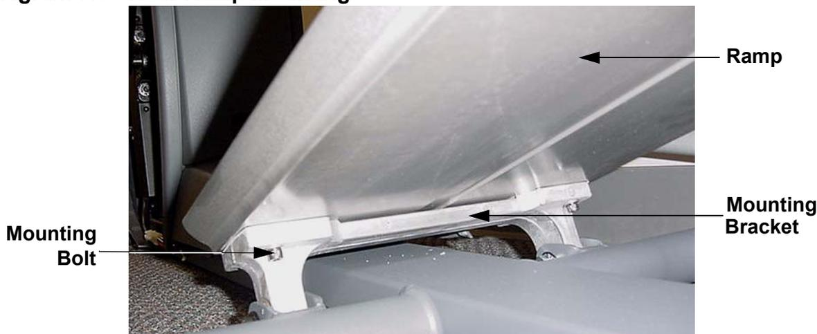
5. Remove the ramp from the EFX.
